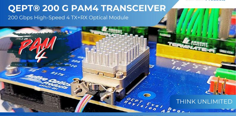
Amphenol AOP QEPT® 200 Gbps PAM4 4 TX+RX High-Speed Optical Module is a robust Quad Embedded Pluggable Transceiver - an ideal form factor to optimize datacenter or supercomputing architectures, thanks to its density and versatility. Supports 200 Gbps across 4 channels (56 Gbps PAM4/channel), it is hot-pluggable and quick to install, a drop-in replacement for the NRZ version.
