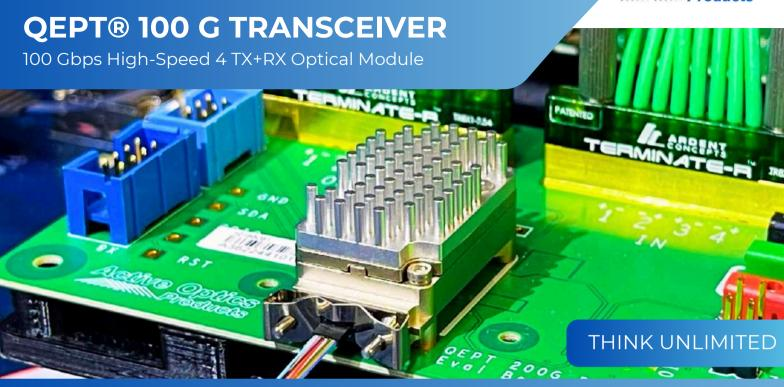
Amphenol AOP QEPT® 100Gbps NRZ 4 TX+RX High-Speed Optical Module is a rugged Quad Embedded Pluggable Transceiver - engineered for extended temperatures and demanding environments where reliability and high performance are crucial. It delivers 100 Gbps across 4 channels (25Gbps/channel), it is hotpluggable and quick to install, a versatile product with a seamless upgrade path to PAM4 56Gbps/channel. specialized space, 8TX or 8RX version are also available.
