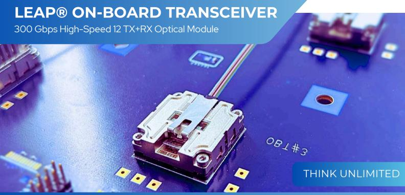
Amphenol AOP 300 Gbps Leap® OBT High-Speed 12 TX+RX Optical Module is faster, smaller, more cost and power efficient than most conventional datacenter interconnects. With its 12 channels working independently and each channel delivering up to 25 Gbps, it is versatile, aggregating up to 300 Gbps. It is the best choice for high density projects that need to take advantage of board space while being as close as possible to the FPGA.
